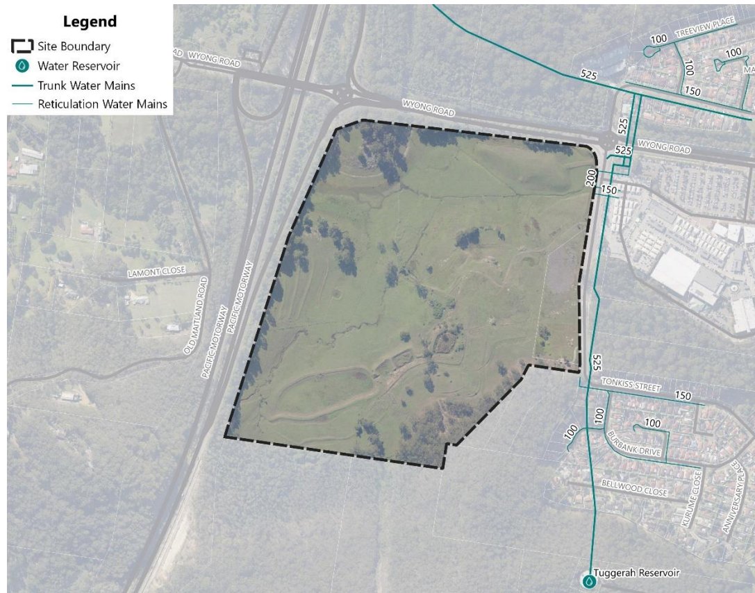
Figure 4 - Existing Water Network
