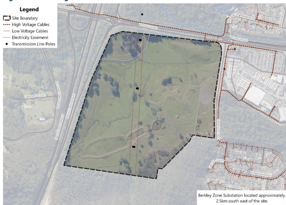
Figure 14 - Existing Electrical Network
