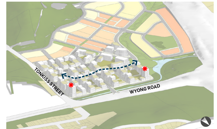
6 Identify two key locations for the highest building height of 12 storeys being: ▪ Mixed use lot eastern bookend - responding to adjoining Westfield. ▪ Mixed use lot western bookends – optimise the amenity of the adjoining Rocky Outcrop. Provide varied heights between these key height markers.
