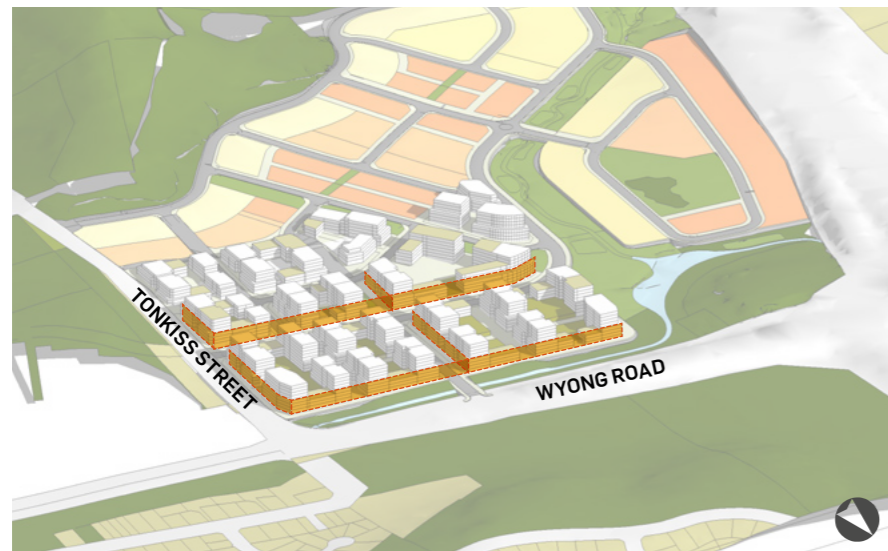
4 Define a four storeys street wall along the main street, Tonkiss St and Wyong Road by adopting an upper-level setback to the apartment buildings.
