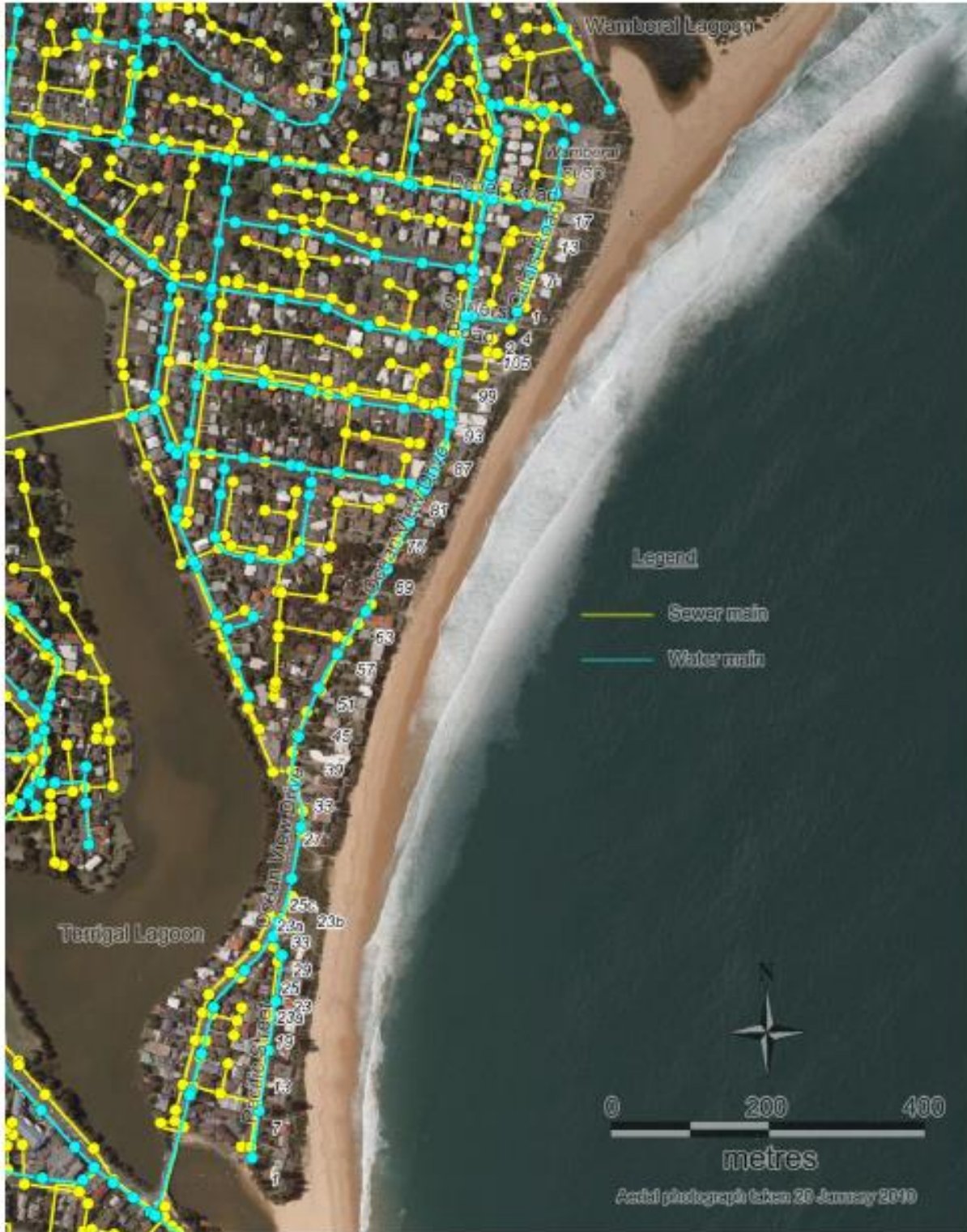
Figure 9.3 Sewer and water infrastructure (WP, 2017, Figure 9)
