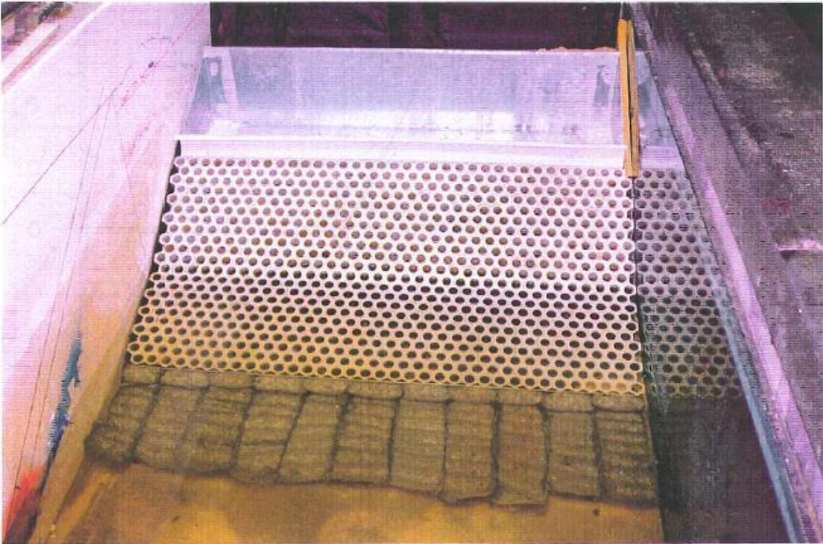
Figure 4.12 Overhead view of Seabees in flume
